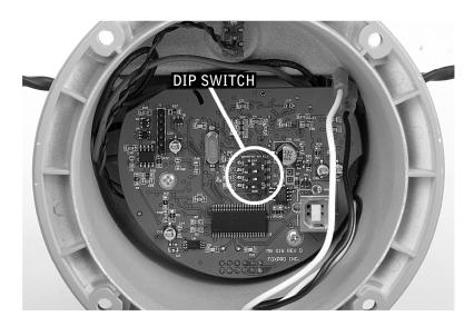
Each of the four switches are marked 1-4. When referring to matrix below, be sure that you modify the switches starting with 1 then continuing on through number 4.
