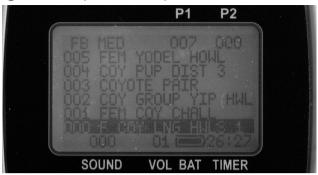
The TX9 features two presets. Each preset provides you with one button access to your most frequently used sounds. The stored sound number of each preset is show in the right corner of the top status line (see image below).
