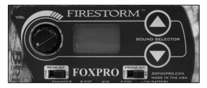
To re-enable the speaker later, simply place the slide switch back to the "ON" position. By disabling the internal speaker(s) when using an external speaker(s), battery life will be extended longer than having all the speakers operating at once.
