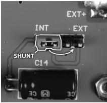
With the shunt connecting the first two pins, audio is routed to the internal speaker only. By
