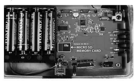
After connecting the micro SD memory card to your computer, the utility should recognize the device as being a valid product and display "Connected to Scorpion X1C." The "Caller Sound Files" column will activate and display the sounds currently installed.
