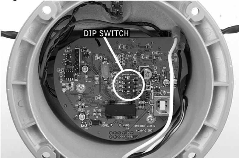
Each of the four switches are marked 1 – 4. When referring to matrix below, be sure that you modify the switches starting with 1 then continuing on through number 4.
